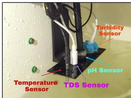
**Figure 2.** Temperature, TDS, pH, and turbidity sensors setup for the system
