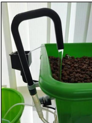
**Figure 5.** Water flow from fish tank to the plant tray and automatic fish feeder
