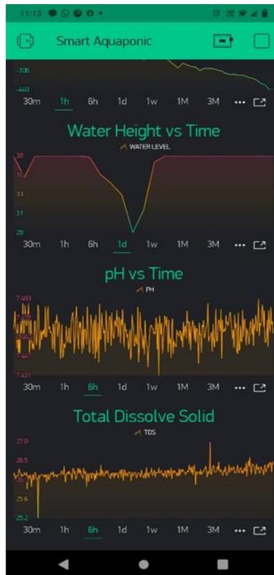
Figure 8. Real time data on mobile using Blynk apps
