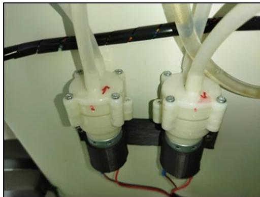
**Figure 4.** Pumps for changing water
