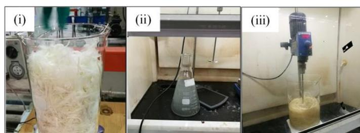
**Figure 2.** i) Weighing of cleaned chicken feathers, ii) Preparation of 1M NaOH solution, iii) Stirring of chicken feathers in NaOH solution
