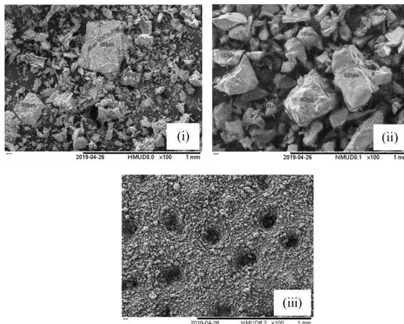
**Figure 12.** Morphology at 100× magnification of keratin powder using (i) Freeze drying (ii) Vacuum oven drying (iii) Spray drying
