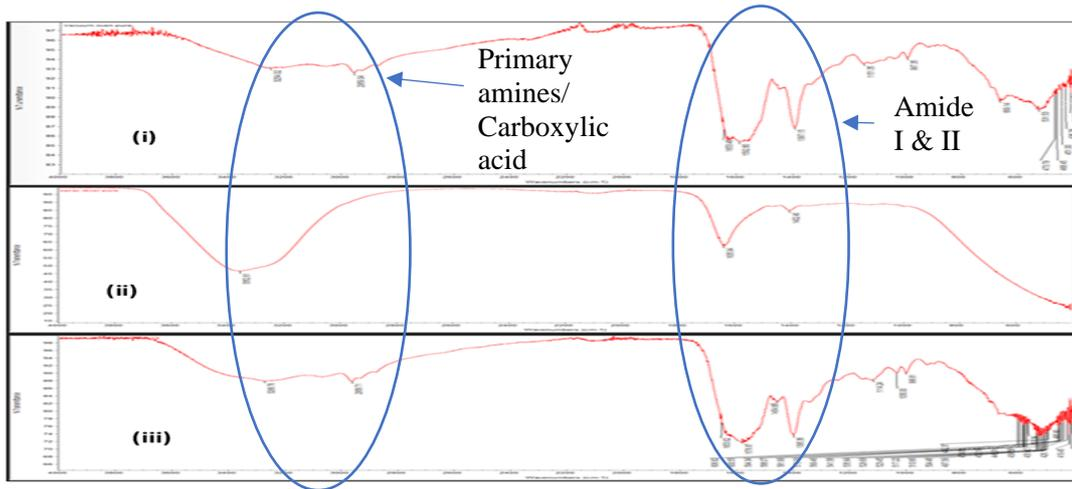
**Figure 10.** Spectrum wavelength of pure keratin powder after (i) Vacuum oven drying at 60°C (ii) Spray drying at 110°C (iii) Freeze drying -80°C
