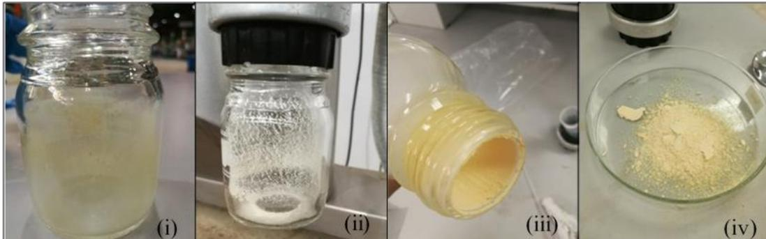
**Figure 8.** (i) Pure keratin powder after spray drying at 60°C, (ii) Keratin-Arabic gum powder after spray drying at 60°C, (iii) Pure keratin powder after spray drying at 110°C (iv) Keratin-Arabic gum powder after spray drying at 110°C
