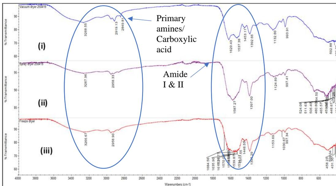
**Figure 11.** Spectrum wavelength of keratin-Arabic gum powder after (i) Vacuum oven drying at 60°C (ii) Spray drying 110°C (iii) Freeze drying -80°C
