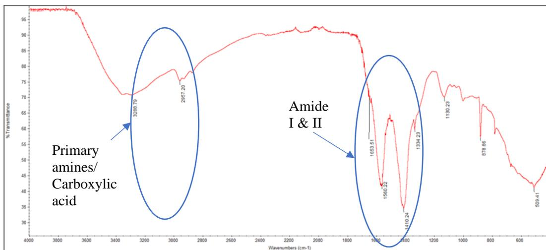
**Figure 9.** Spectrum wavelength of keratin solution before drying
