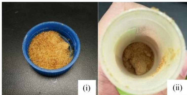
**Figure 7.** Physical appearance of (i) Pure keratin powder after placing in oven for 24 hours (ii) Keratin-Arabic gum powder after placing in oven for 24 hours
