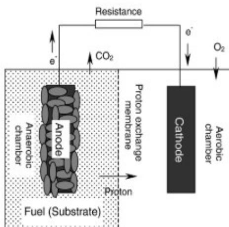
Figure (2) General schematic diagram of two chambered MFC (Du et al., 2007)
