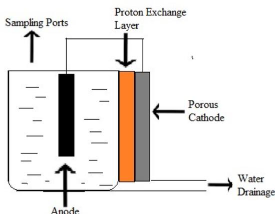
Figure (3) Schematic diagram of single chambered MFC (Park and Zeikus, 2003)
