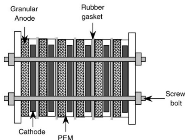
Figure (4) Stacked MFC configuration of 6 individuals units with granular graphite anode (Aelterman et al., 2006).
