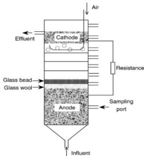
Figure (5) Up-flow MFC reactor configurations (Du et al., 2007).
