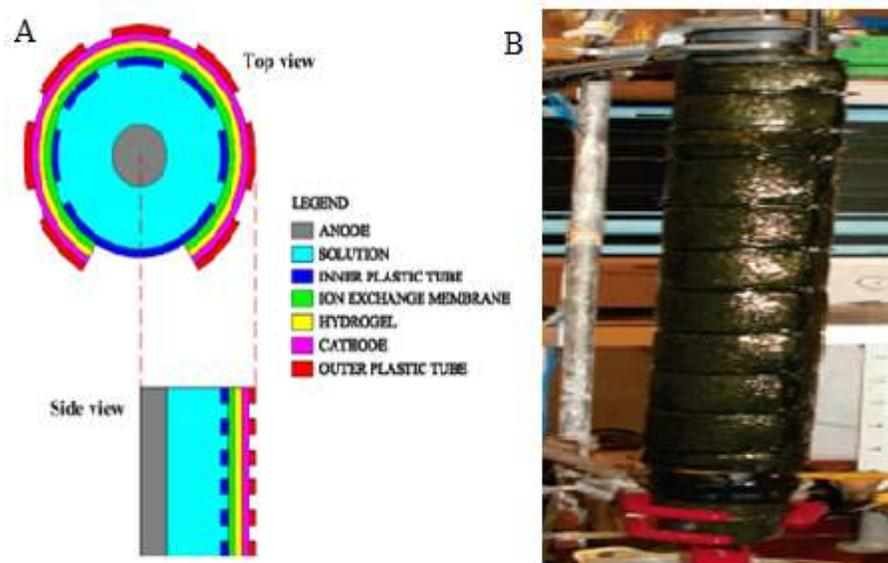
Figure (6) A) Schematic Diagram of tubular MFC (top and side view) (Kim et al., 2009). B) Up-flow tubular MFC with inner graphite bed anode and outer cathode (Logan et al., 2006).
