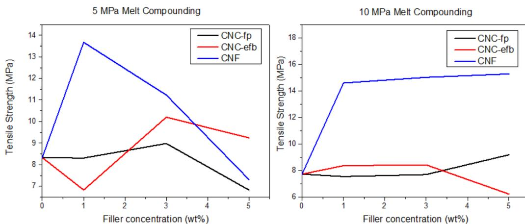
Figure 4. Tensile strength of the recycle paper at different nanocellulose loading.
