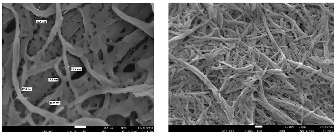
Figure 1. (Left): FESEM image of CNF under 90 kX magnification (Reproduction of image from John Wiley & Sons Ltd with permission from Yahaya et al., Synthesis of Active Hybrid Films Reinforced with CNF as Active Packaging Material 2022; 45: 8: 1448-53[14] and Figure 2. (Right): CNC-fp image under 50 kX magnification.
