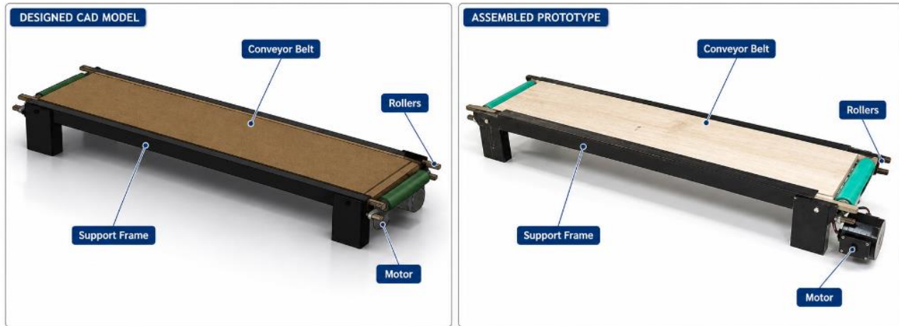
Figure 3. Comparison of the designed CAD model and the assembled conveyor-belt prototype
