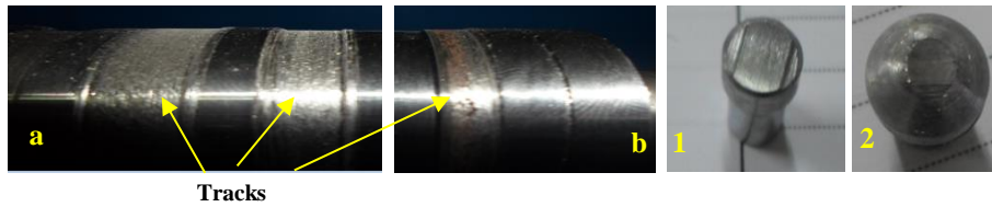
Figure 8. Cylinder and pins track after tribology: (a) and (1) Dry contact, (b) and (2) Lubricated contact
