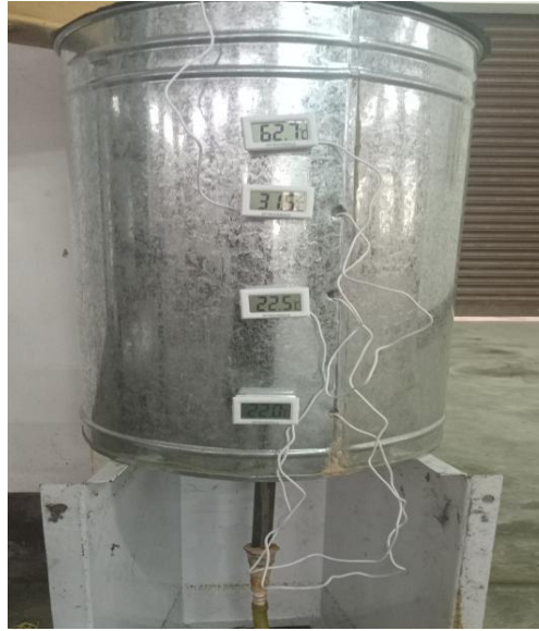
Figure 2. The in-house designed and fabricated TES system
