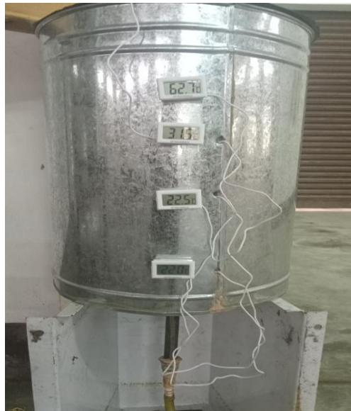
Figure 2. The in-house designed and fabricated TES system
