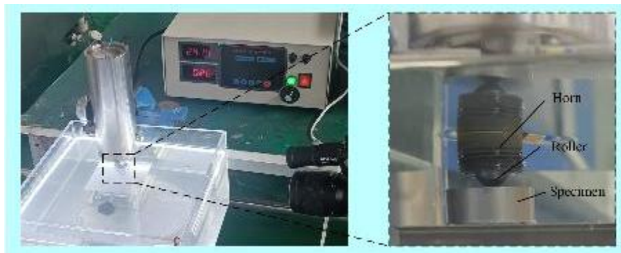
Figure 3. Ultrasonic cavitation experimental device
