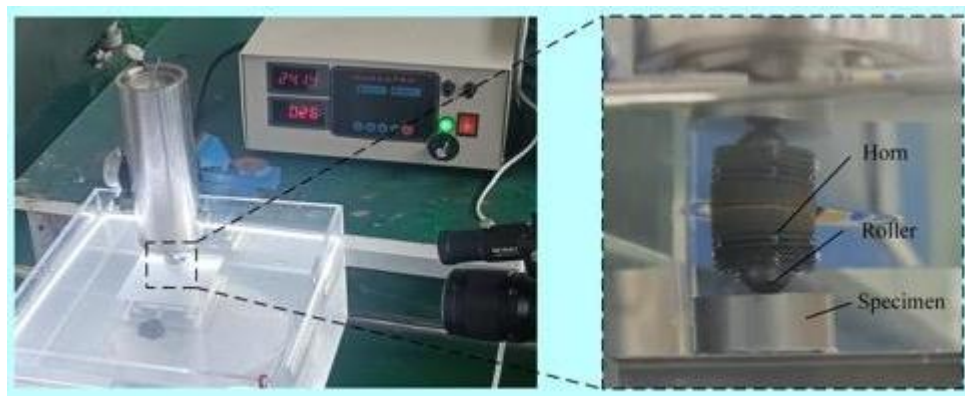
Figure 3. Ultrasonic cavitation experimental device
