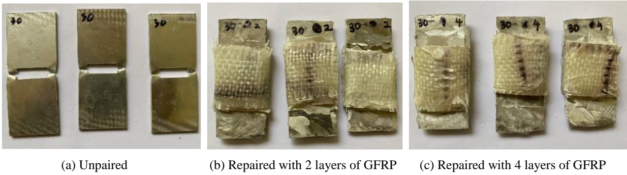
Figure 10. Edge-cracked specimens with a crack length of a = 15 mm: (a) unrepaired, (b) repaired with 2 layers of GFRP, and (c) repaired with 4 layers of GFRP
