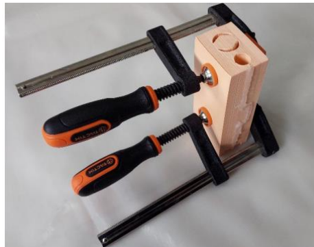
Figure 4. Mould assembly secured with clamps prior to injection
