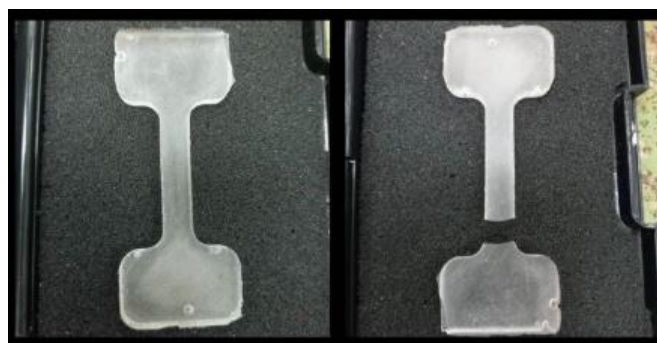
Figure 8. (Left) Test sample of silicone Sylgard 184; and (Right) test sample after the tensile experiments
