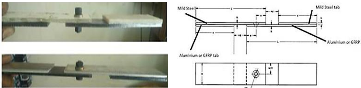
Figure 6. Specimen test using single-bolted joints [49]
