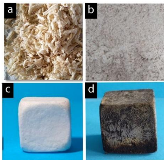
Figure 2. Digital images of (a) cleaned and dried sugarcane bagasse, (b) ground sugarcane bagasse, (c) MFC foam, and (d) mCNT-MFC foam
