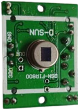
Figure 1. PIR Sensor Module
