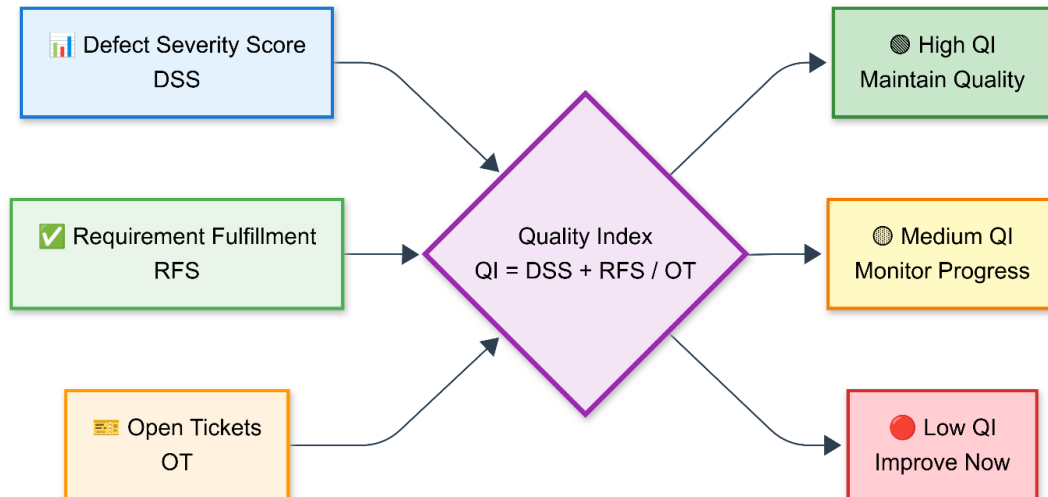
Figure 3. Defect Density Quality Measurement
