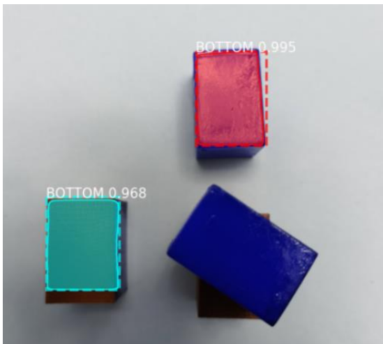
Figure 7. Part of the target object was not identified
