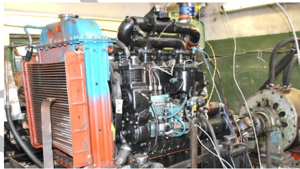
Figure 1. View of the D-243 engine on the test stand
