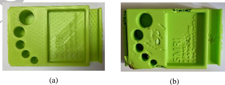
Figure 2. The example of AM product where (a) non-defect product; and (b) defect product
