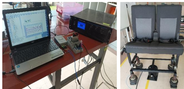
(a) vibration transmissibility setup
