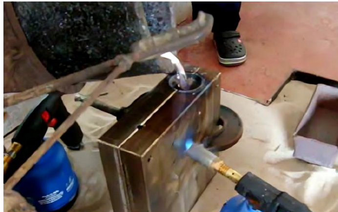
Figure 6. Pouring process at 900 °C for the vertical orientation mould
