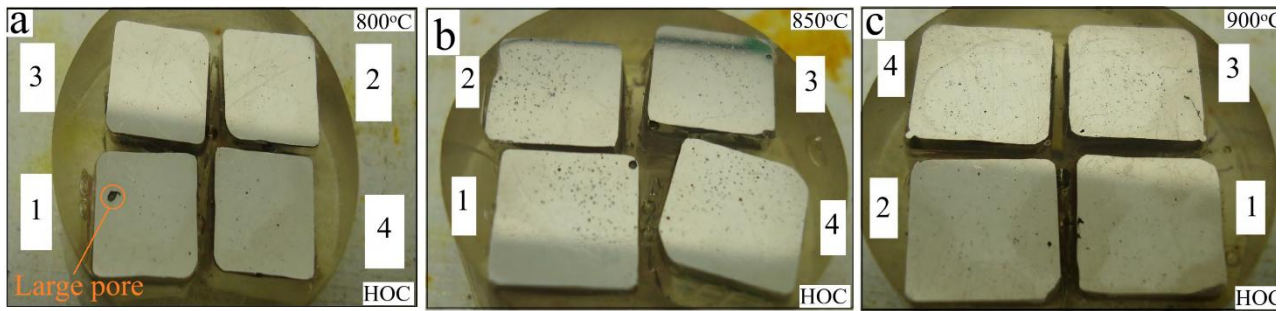
Figure 13. Visual inspection of macro-porosity at the cross-section of HOC castings at different pouring temperatures; (a) at 800 °C, (b) at 850 °C, and (c) at 900 °C
