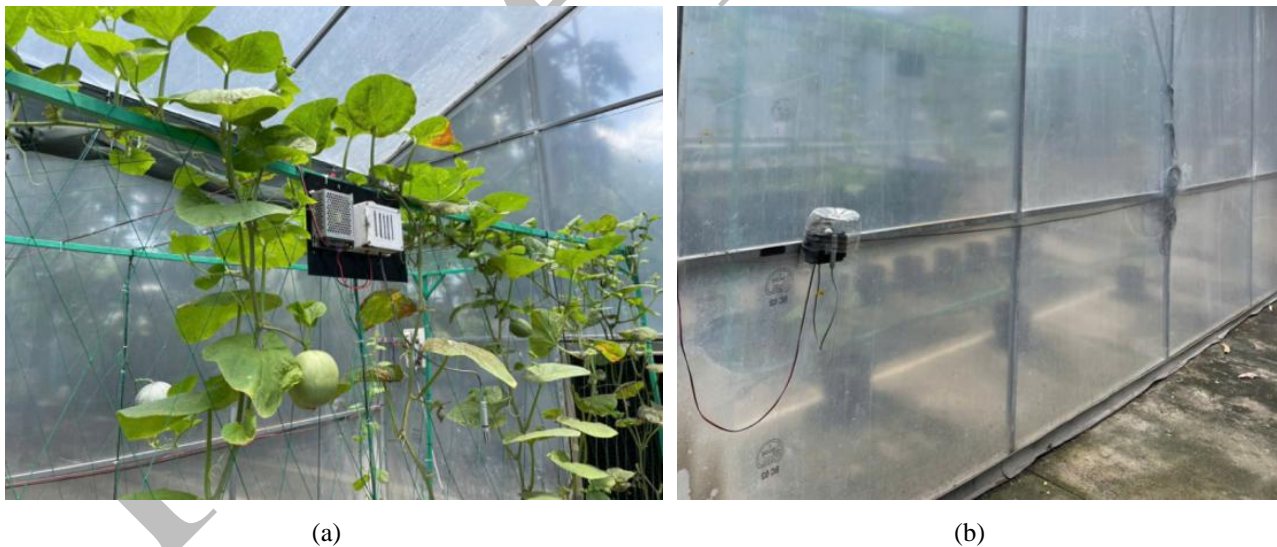
Figure 13. Sensor installation locations for greenhouse environmental monitoring: (a) inside the greenhouse; (b) outside the greenhouse
