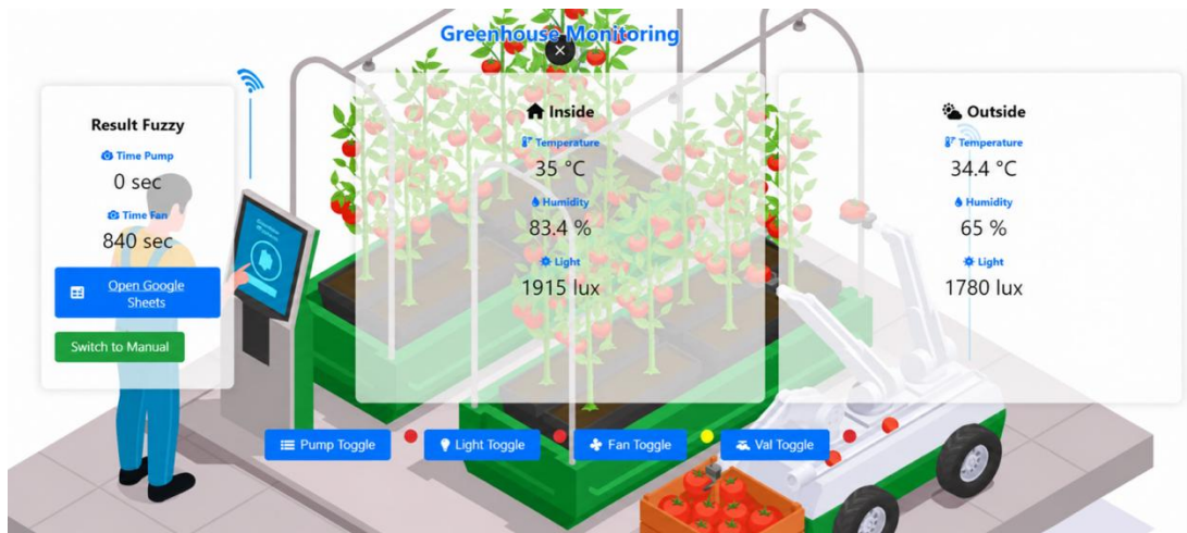
Figure 15. Web-based monitoring and control interface
