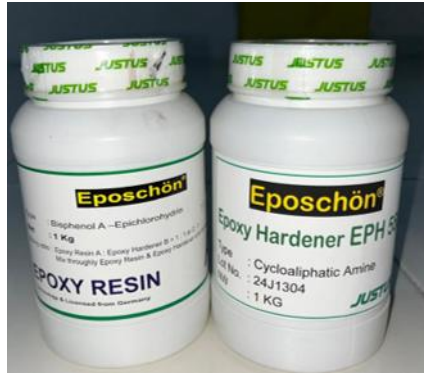
Figure 2. Bisphenol A-Epichlorohydrin epoxy resin and Cycloaliphatic Amine type hardener epoxy
