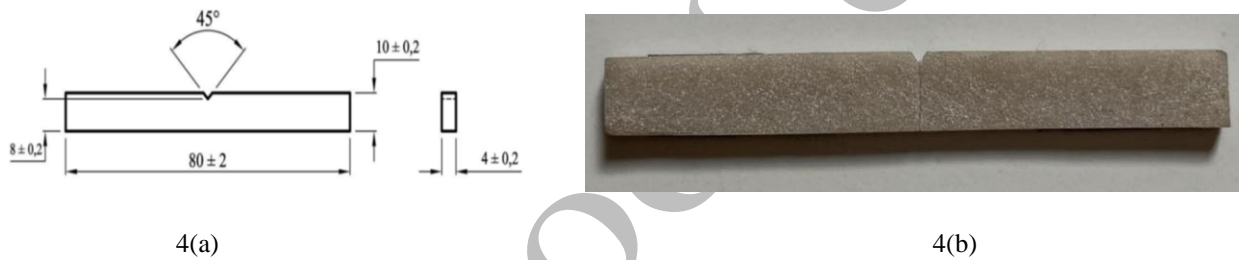
Figure 4. (a) Standard dimension for Impact test (ISO 179-1), (b) Impact test specimen
