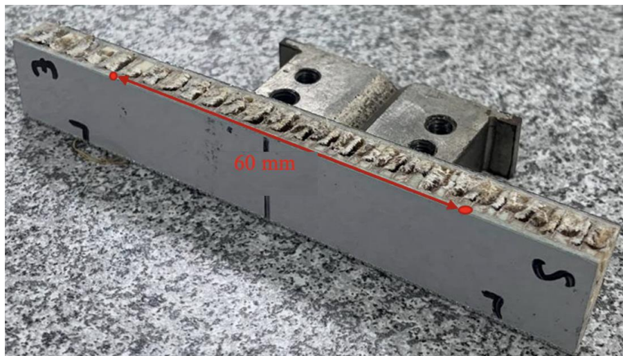
Figure 6. Surface roughness measurement procedure used in this study
