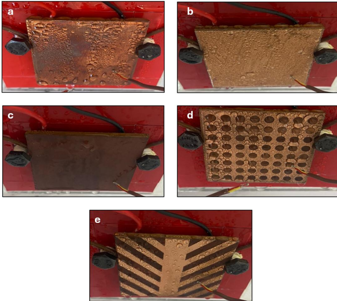
Figure 6: Condensate formation on (a) Untreated (b) PVC-coated (c) laser etched (d) desert toktokkie beetle spot pattern, and (e) leaf vein skeleton pattern samples
