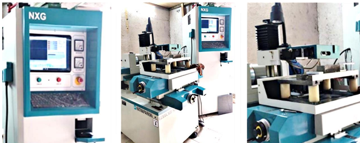
Figure 3. Image of a wire-cut machining using electrical discharge apparatus
