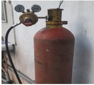
(a) Hydrogen supply cylinder with dual-stage pressure regulators
