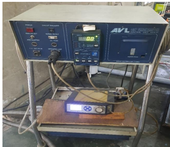
Figure 3. AVL DIGAS 444 Exhaust Gas Analyzer and 437 Smoke Meter used for emissions measurement
