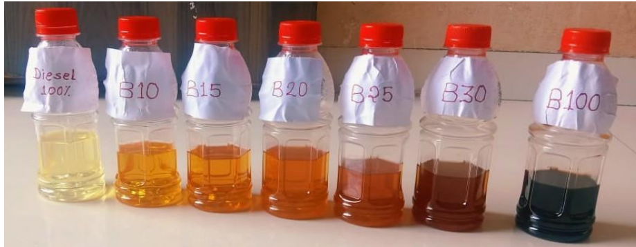
Figure 1. Pure diesel and Neem biodiesel blend samples were used in experimental testing
