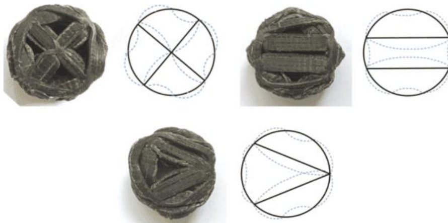
Figure 10. Deformation modes for multicell constituent elements
