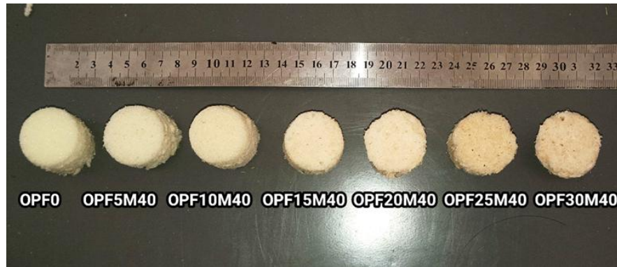
Figure 4. Samples prepared for sound absorption test
