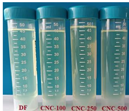
Figure 4. Actual image of diesel fuel and nanofuel samples at the end of the two hours
