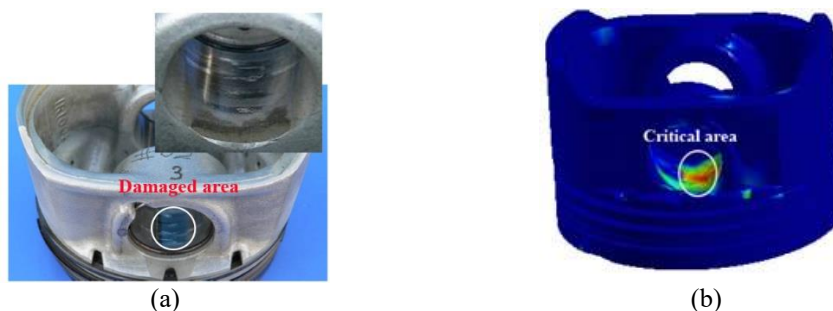
Figure 15. (a) The ruptured piston in real condition [43] and (b) the critical area of the present study
