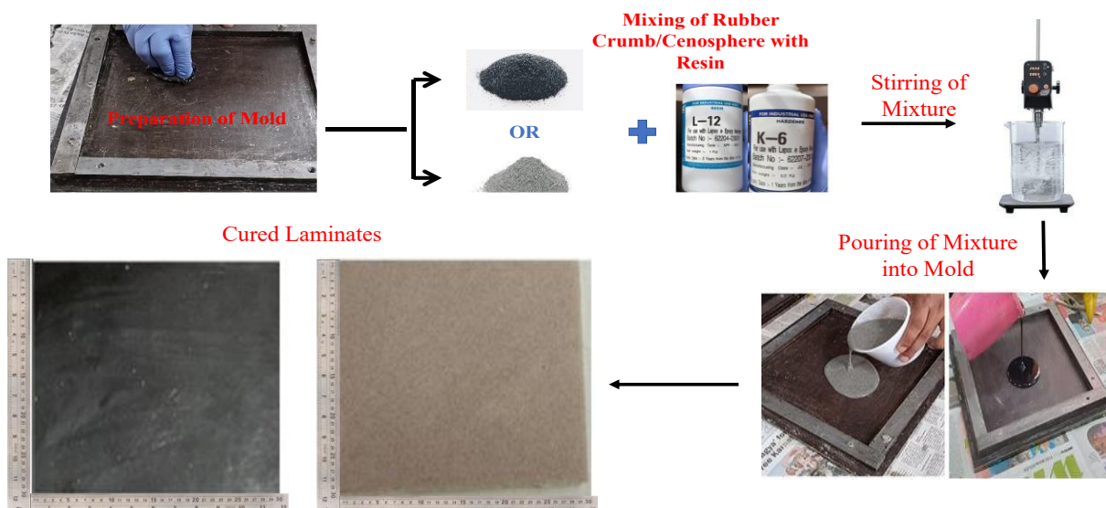
Figure 2. Steps involved in preparation of syntactic foams
