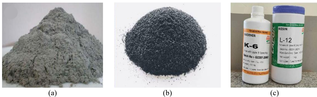
Figure 1. Raw materials utilized for production of syntactic foams: (a) cenosphere; (b) rubber crumb; (c) epoxy matrix
