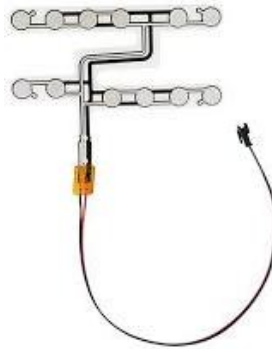
Figure 8. Inductive seat occupancy detection sensor
