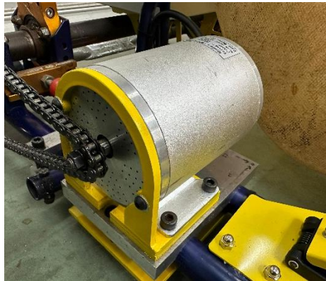
Figure 2. 1,800W DC motor for the go-kart
