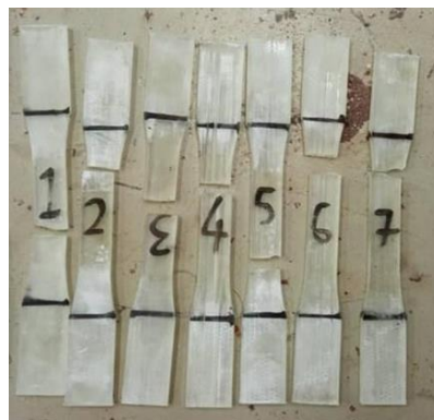
Figure 13. Condition of specimens after tensile test for the PLA resin specimen
