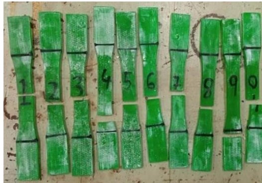
Figure 12. Condition of specimens after tensile test for the ABS resin specimen
