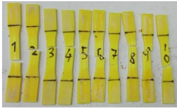
Figure 11. Condition of specimens after tensile test for the ABS filament specimen
