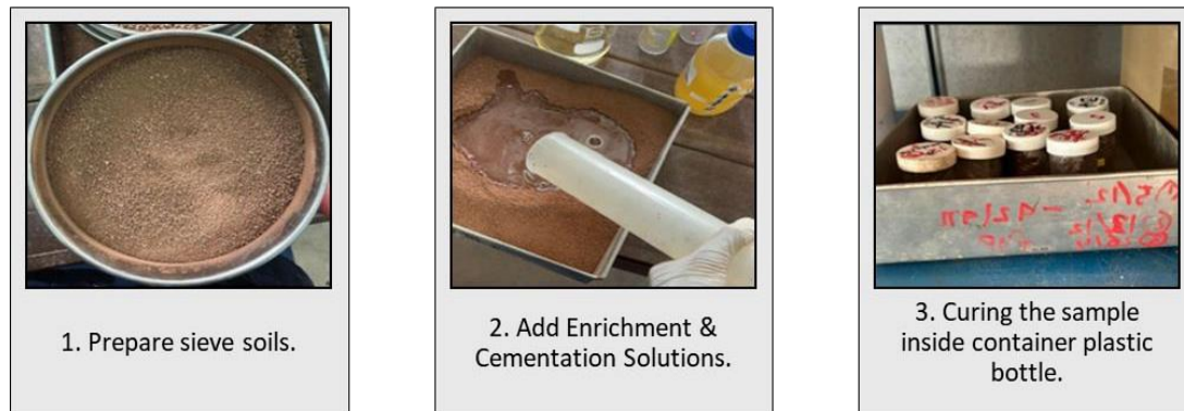
Figure 4. Sample preparation for UCS test
