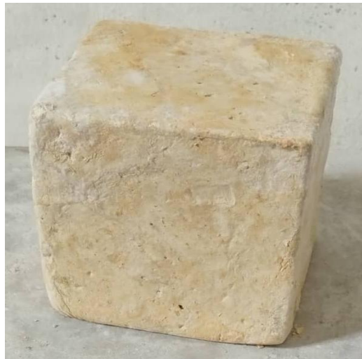
Figure 4. Sample of kenaf fiber - soil reinforced block
