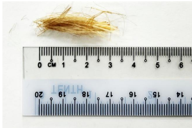
Figure 3. Sample of kenaf fiber (standardized at 30 mm to 50 mm in length)
