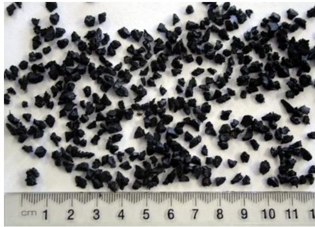
Figure 2. Sample of crumb rubber tire waste materials (1 to 4 mm and 5 to 8 mm size)
