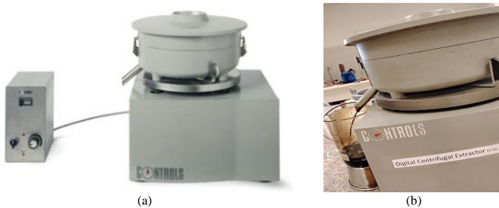
Figure 4. The process of removing asphalt binder from RAP (a) asphalt binder centrifugal device, (b) separation of asphalt binder)
