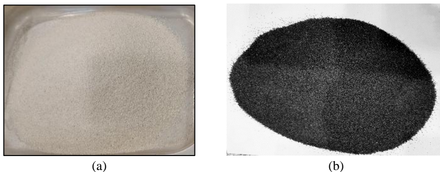
Figure 2. Fine aggregate utilized in the same single size (a. feature of quartz sand, b. feature of magnetite black sand)
