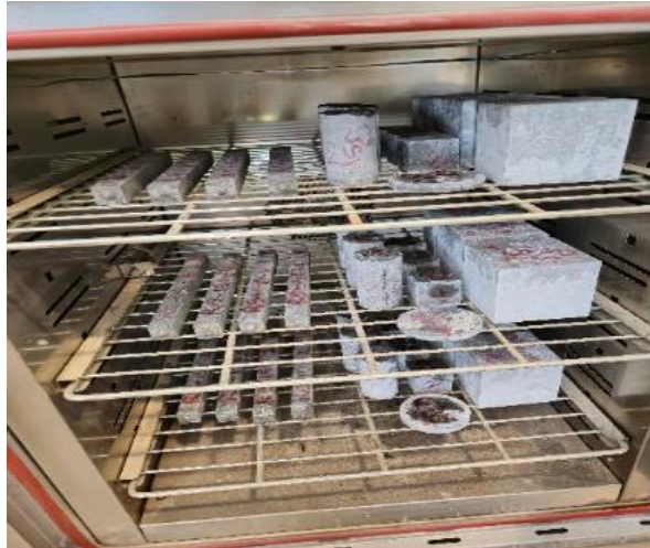
Figure 8. Very-high strength heat-resistant concrete samples in oven
