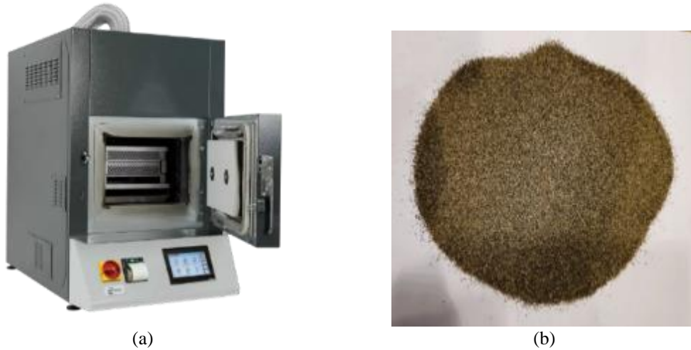
Figure 5. Process of preparing recycled asphalt pavement aggregate by ignition method (a) asphalt binder analyzer device, (b) recycled asphalt pavement aggregate)
