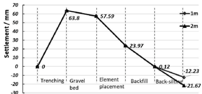
(c) Vertical displacement of the tunnel
