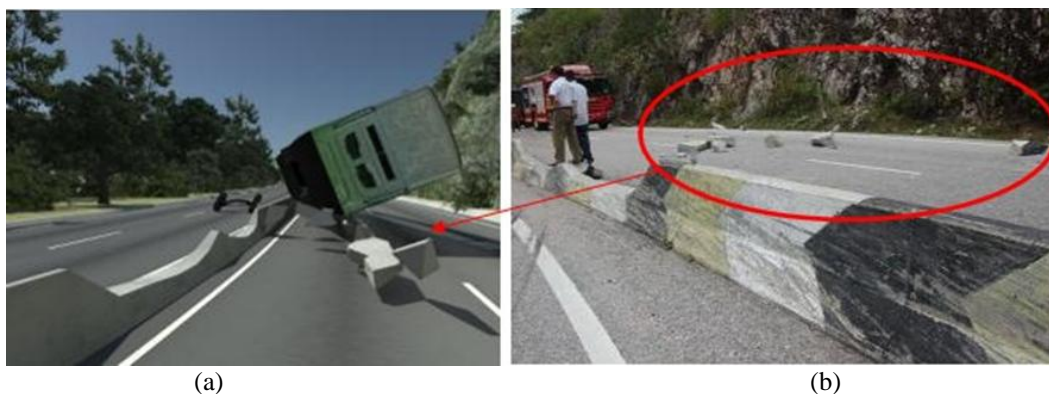
Figure 2. (a) The crash involving an express bus, (b) The front axle detached after colliding with a concrete barrier
