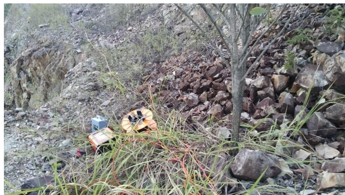
Figure 3. Setting up of electrical resistivity mapping apparatus on the site
