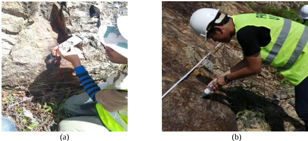
Figure 2. Field mapping of slopes. (a) Scanline mapping (b) Measurement of surface hardness of rock surface using Schmidt Rebound Hammer
