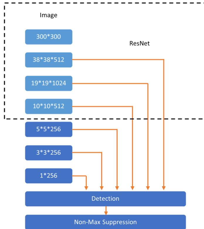
**Figure 1.** Face detection model based on SSD-ResNet [14].
