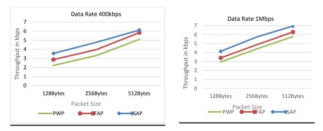
Figure 17. Throughput vs. packet size DR=400kbps Figure 18. Throughput vs. packet size DR=1 Mbps
