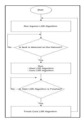
Figure 1. Proposed Model for Single and Multi-Fault Tolerance
