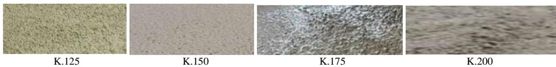
Figure 1. Concrete image with various strength levels
