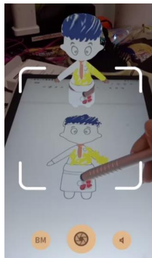
Figure 11. When the user applies colors to the marker, the marker with the customized look will be mapped to the texture of the AR avatar in real-time
