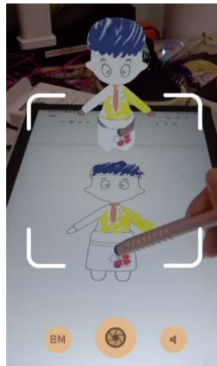
Figure 11. When the user applies colors to the marker, the marker with the customized look will be mapped to the texture of the AR avatar in real-time
