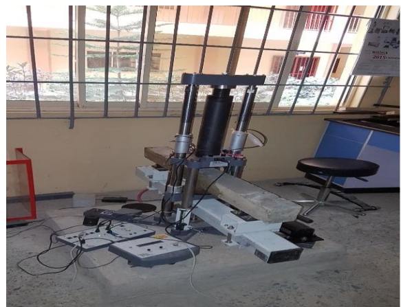
Figure 6. Flexural testing of sample beam
