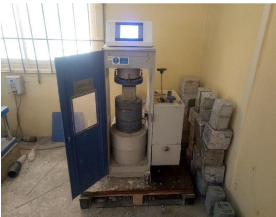
Figure 5. Compression testing machine in action
