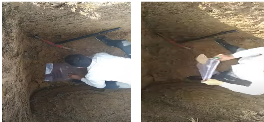
Figure 9: Site Photography showing sampling inside Trial Pit
