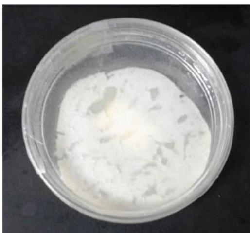
**Figure 3.** Phase separation of F4 at temperature  $45\text{ }^{\circ}\text{C} \pm 70\%$  RH for 48 hours.
